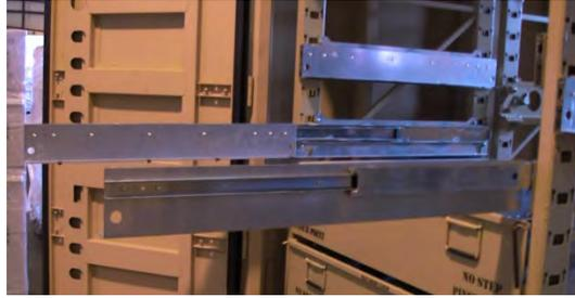
18. Position drawer on the slide ledge being careful to align mounting holes.
