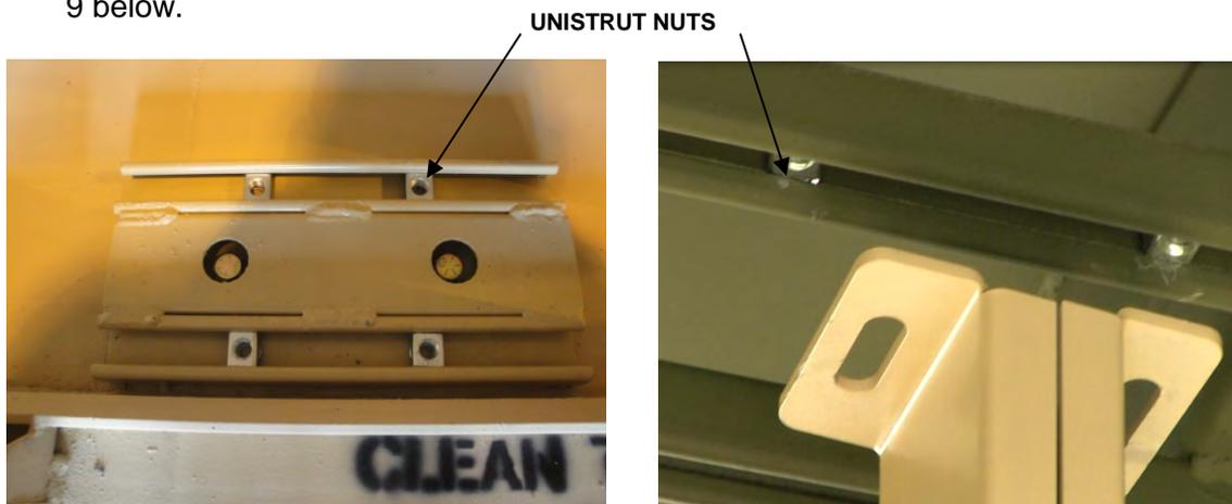
3. Install (4) vertical rack frames to base plates with (8) ½" lock washers, (8) ½" flat washers and (8) 1-inch bolts. Apply Locktite 262 to bolt threads and hand tighten only.
