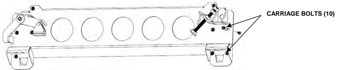
11. Place the pallet ledges in their desired positions by inserting the bayonet tabs into the vertical rack frame windows while aligning the ten carriage bolts into their appropriate slots.
