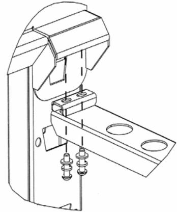
18. Install front pallet ledge stabilizer with the four Button Head Bolts with 5/16-inch lock washers using 3/16-inch hex driver socket and 3/8-inch ratchet with extension from the two positions of each pallet ledge. There are four bolts located at each vertical rack frame.
