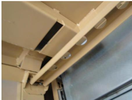
17. Install rear pallet ledge stabilizer with four Button Head Bolts with 5/16-inch lock washers using 3/16-inch hex driver socket and 3/8-inch ratchet with extension from the two positions of each pallet ledge. There are four bolts located at each vertical rack frame.
