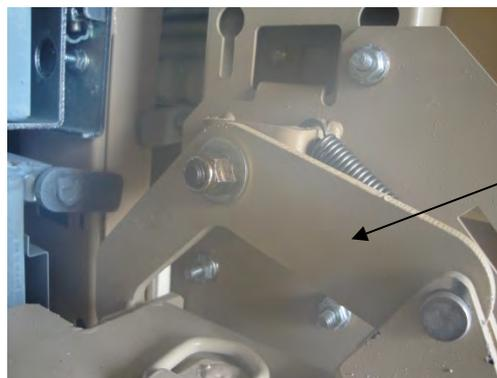
29. Tighten jam nut using 7/8-inch combination wrench to hold lock rod in the closed position.
