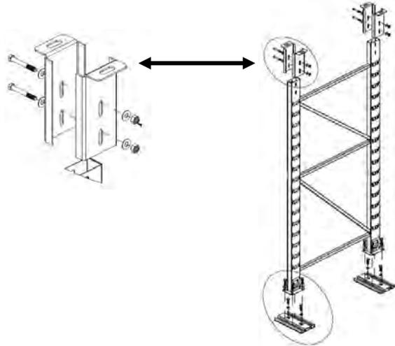
5. Secure upper sleeves to ceiling mount using (4) 1-inch bolts, (4) ½-inch lock washers, and (4) ½-inch flat washers. Apply Loctite 262 to bolt threads and hand tighten only.
