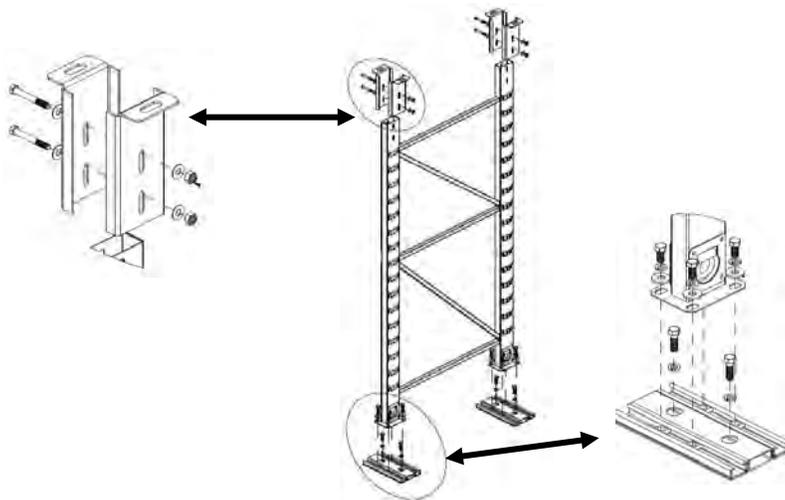
19. With someone holding the vertical rack frame, remove the 1/2-inch hex head bolts and washers from the top (2) and bottom (4) mounting plates using a 3/4-inch socket with ratchet.
