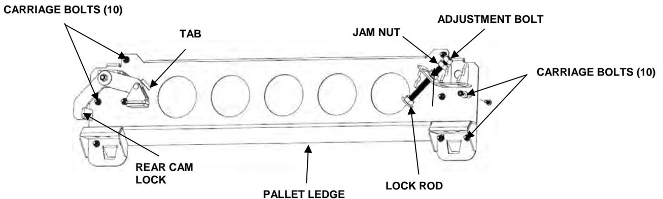
15. Pallet ledges are retained on the vertical rack frame by ten 1/4-inch carriage bolts and four bayonet tabs protruding into the windows of the vertical rack frame. This requires the ledge to be loosened from the vertical rack frame. While one person securely holds the pallet ledge, the second person applies an upward force by tapping the underside of the ledge at the attached point with a 2 X 4 soft wooden block or similar material.
