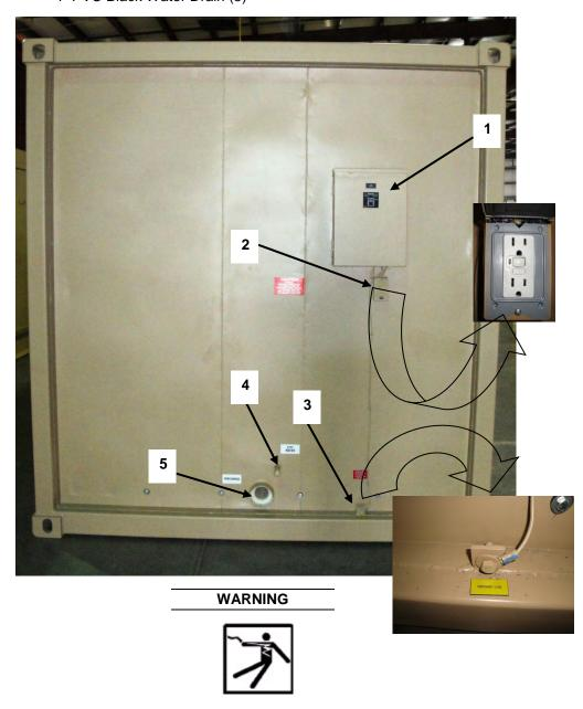
The electrical ground must be established first to prevent electrical shock to personnel. Consult National Electrical Code Section 250.
