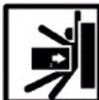
If a container is dropped during transit movement of any kind, extreme care should be taken when opening the doors to preclude material from falling on and injuring personnel.
